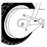
**9** Re-attach the chain guard. Test ride and check. Readjust as needed.
